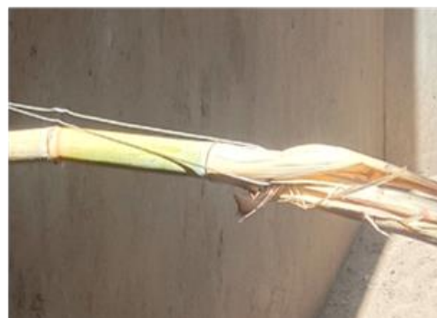
Fig. 4. Measurement the force required for removing sheath and leaves.
