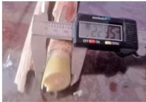
Fig. 3. Sugarcane stalk diameter measuring at three different positions.
