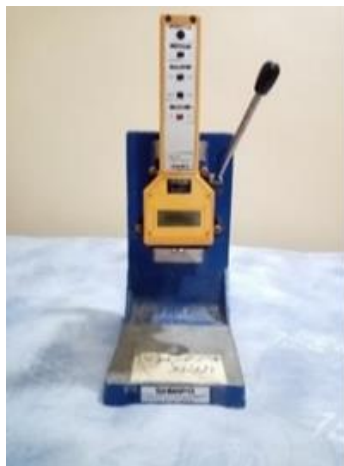
Fig. 1. Digital force gauge models DF-FG 5, and apparatus designed by (Zaalouk and Ghanem, 2003).
