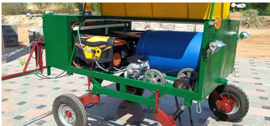
Fig. 10. Isometric view of the spraying machine shows the power supply system.
