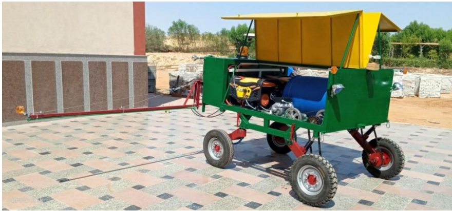
Fig. 3: The spraying machine with opening machine cover.
