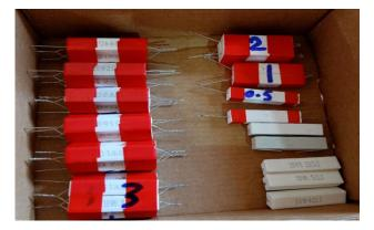
Fig. 5. The power resistors.
