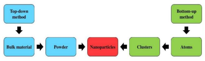
Fig. 2: The nanoparticles synthesis process.
