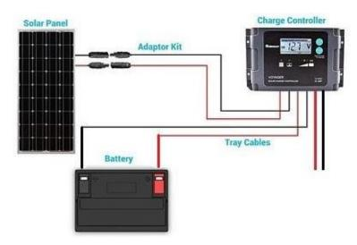
Fig. 4. PV system diagram.
