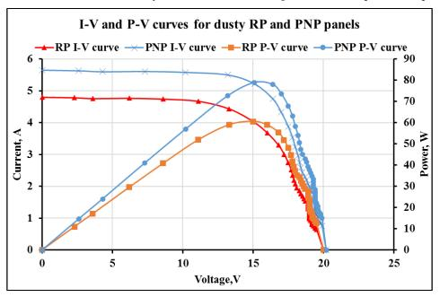
Fig. 12. The I-V and P-V curves for dusty RP and PNP.
