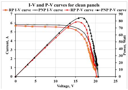
Fig. 7. The I-V and P-V curves for clean RP and PNP.
