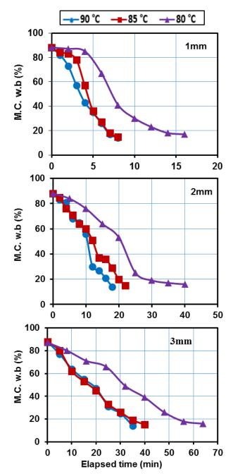
**Fig. 2.** Moisture contents wet basis (%) of Guava puree as affected by water basin temperature and drying elapsed time at the three different thicknesses studied.
