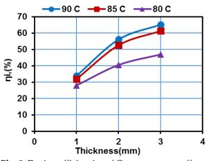
**Fig. 8.** Drying efficiencies of Guava puree as affected by puree thickness, water basin temperatures.
