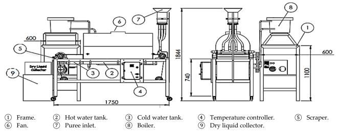
Fig. 1. Elevation and side view of (RW) dryer structure.
