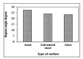
**Fig. 6.** Angle of repose for white Mulberry fruits on different material surface.
